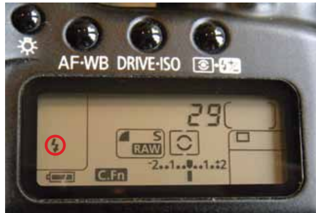
Figure 7: The miniature lightning bolt signifies that the white balance is set for flash operation.
