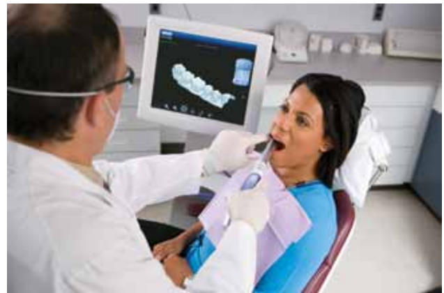
Figure 4: Lava chairside oral scanner (3M ESPE; St. Paul, MN). Lava "3D-in-motion" technology allows the dentist to capture and simultaneously view continuous 3D video images to create a digital impression. The system is flexible for prescribing porcelain-fused-to-metal and CAD/CAM restorations.
